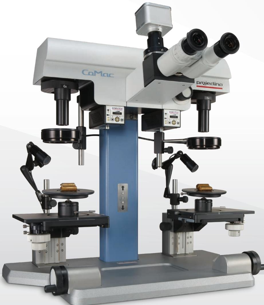
Zoom objectives, assembled on a rotating turret, provide magnification levels from 2.5x to 72x
