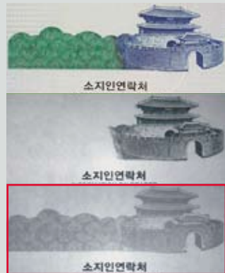
■ Comparative illustration with IR absorption; above: original in visual light, middle: IR 850 nm absorption, below: forgery
