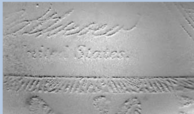
■ Magnetic Ink Detector: Detector to visualize magnetic ink in documents
