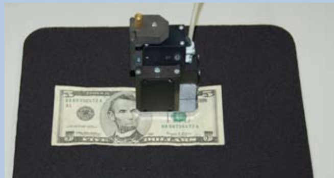
■ Magnetic Ink Detector: Detector to visualize magnetic ink in documents
