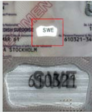
■ MLI Multiple Laser Image Visualization with side light
